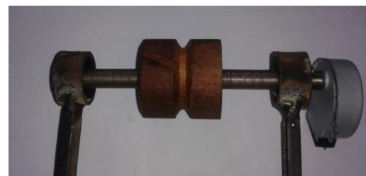
Fig.8: Pulley and Bearing assembly
